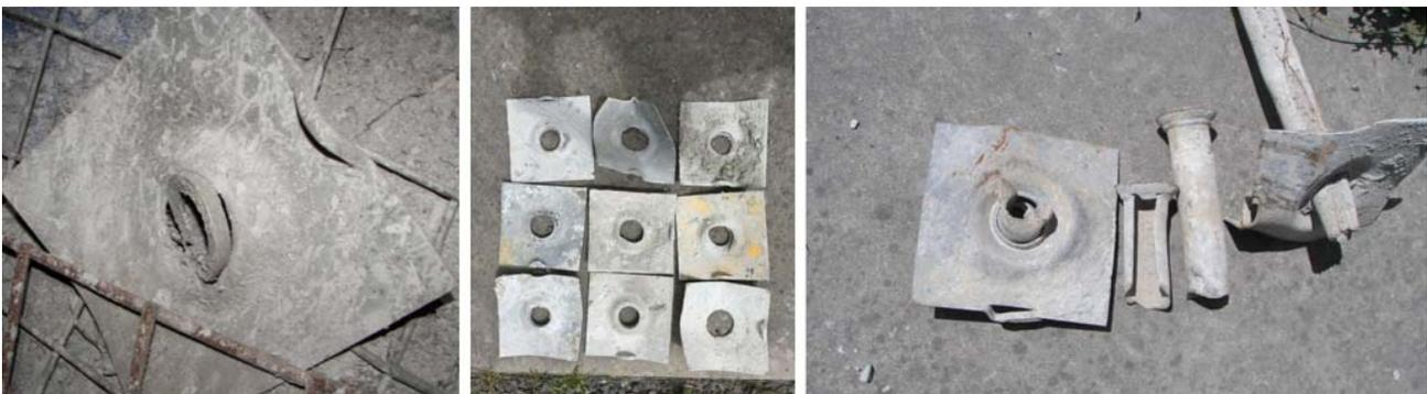
FIG 6 – Friction bolt failure examples
