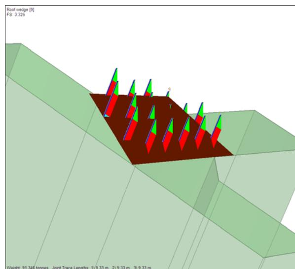
**Figure 5 Output from one 2.4 m grouted bolt design in a normal intersection**
