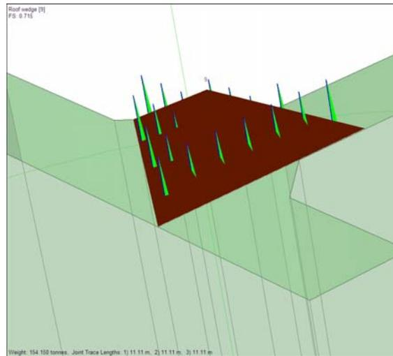
**Figure 6 Output from 2.4 m ungrouted bolts used in an oversize intersection**
