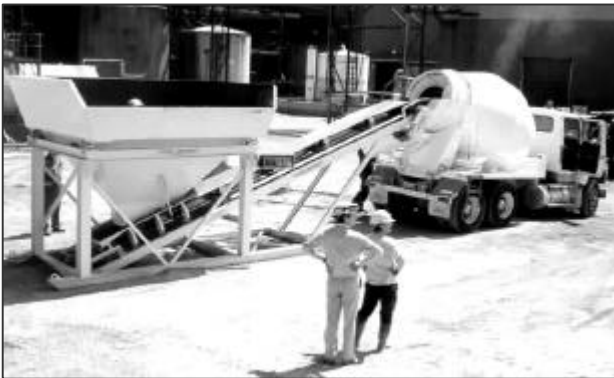
Plate 2. Batch Plant and Agitator
