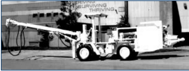
Plate 1. Modified Jumbo based Shotcrete Machine
